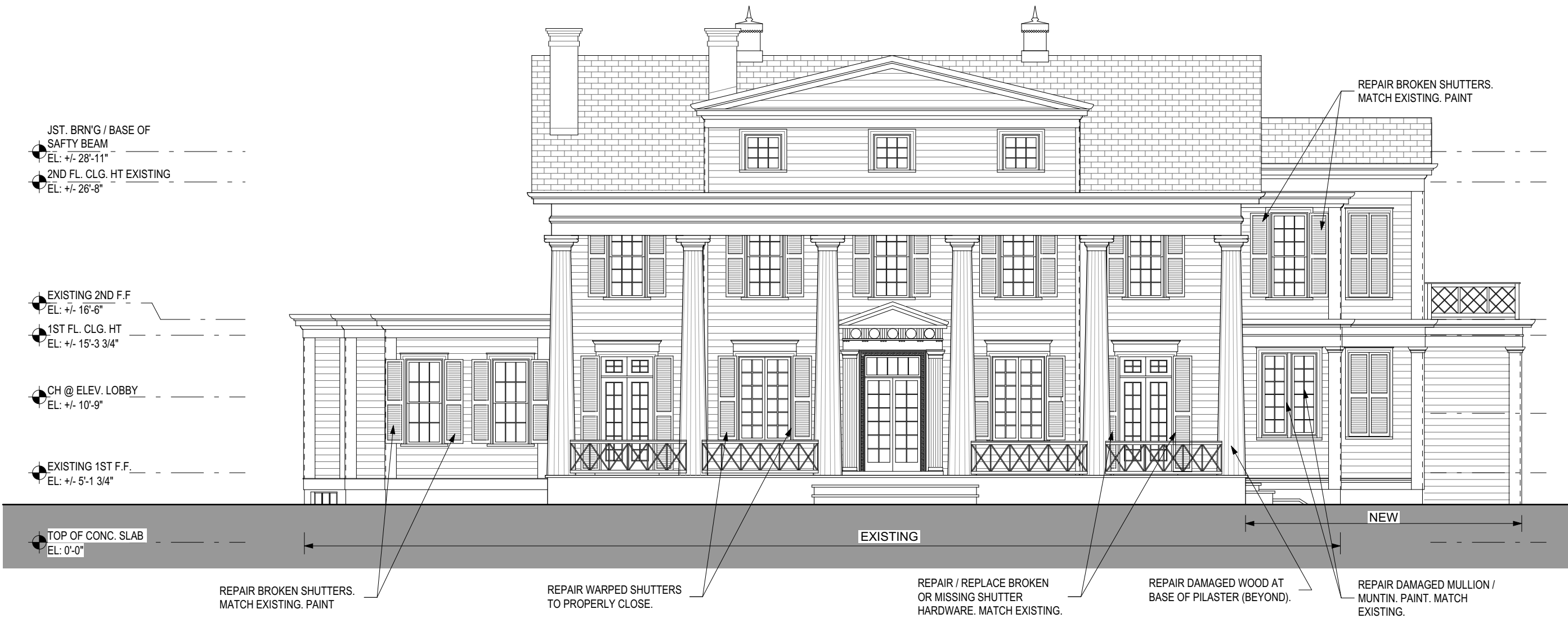
6 OVERALL SOUTH ELEVATION - ADD ALT. No. 4 A6.1 SCALE: 1/8" = 1'-0"
