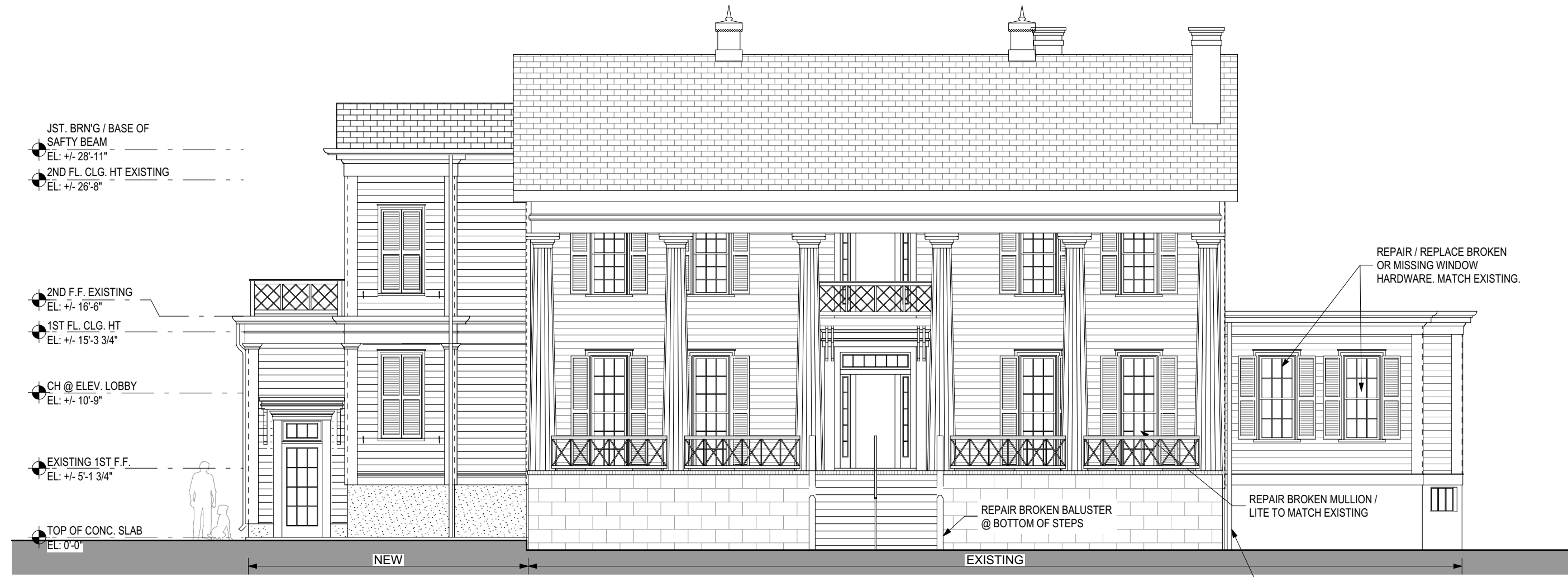
1 OVERALL NORTH ELEVATION - ADD ALT. No. 4 A6.1 SCALE: 1/8" = 1'-0"
